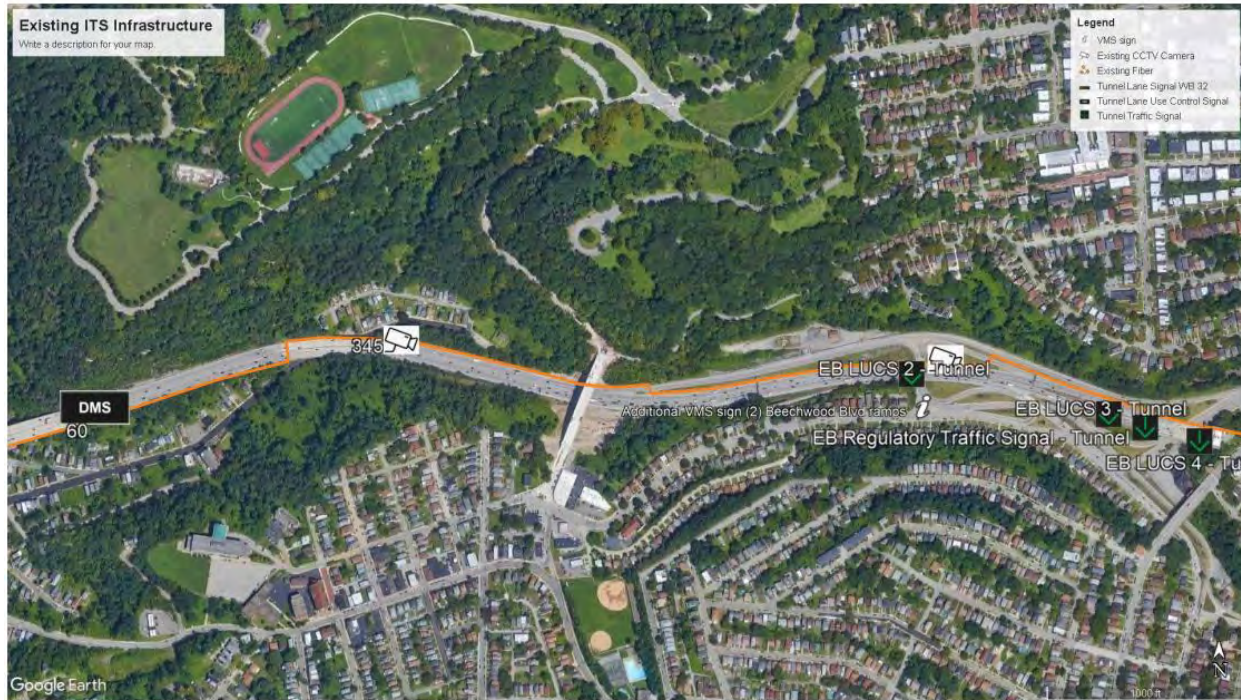
Figure 15: Existing ITS Infrastructure (Larger image in Appendix E)
